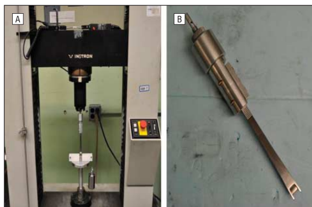
Figure 2. A, The Instron universal tester setup before an osteotome sharpness testing trial. B, Close-up view of the osteotome seated in its specially designed holder.
