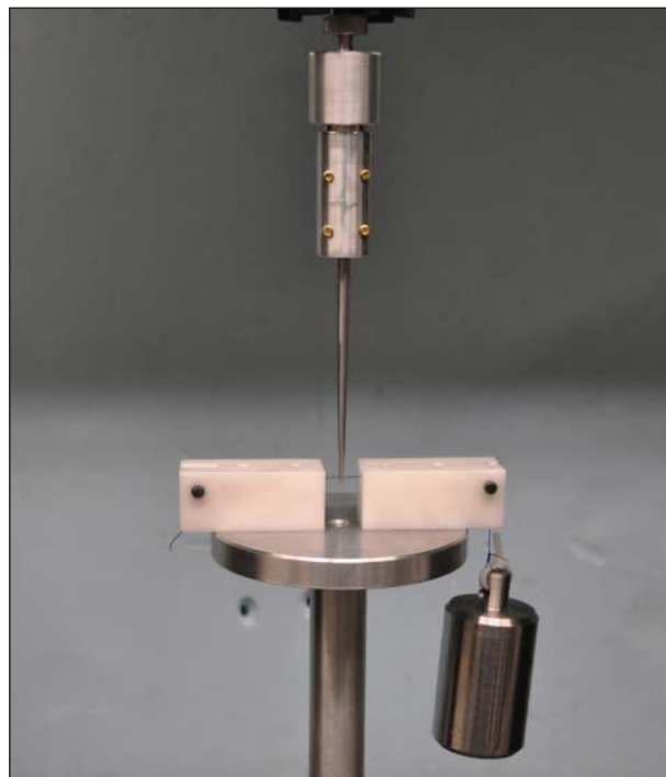
Figure 3. Close-up view of the testing setup and the holders that were created for the osteotomes and the No. 2 monofilament polypropylene suture.
